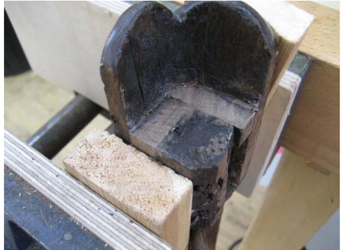
The cross grain peg was trimmed back and sealed with shellac and the small voids stopped with beeswax. After minimal trimming of the mating surfaces walnut splices were glued into the lost areas with hide glue and levelled in to the existing surface.
