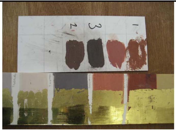
The losses had the ground cleaned before treatment with rabbit skin glue size was applied. The areas were then filled with an acrylic gesso applied with a gilders gesso tool. Each layer was sanded and inspected before levelling with a gilders scraper.
