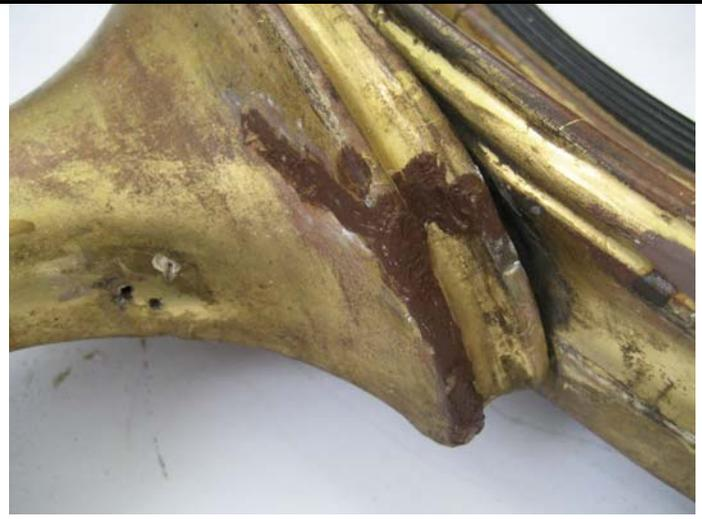
Each successive coat of bole was cut back using silicon carbide paper and the bole was built up to around 5 layers before a pre-gilding burnish. The latter coats were allowed to spread slightly to allow a graduation in the joint facilitating a more suitable edge around the damage.
