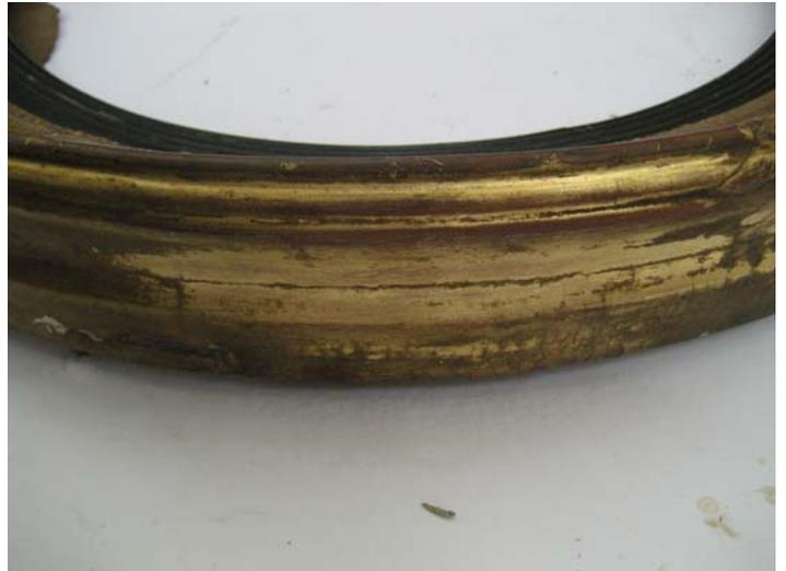
After testing inconspicuous areas to ascertain compatibility it was decided to use cotton swabs saturated in either acetone (for the water gilded areas) or deionised water (for the oil gilded areas) to remove surface accretions and soiling. Around 100 individual buds were used to allow careful control over the amount of debris removed from this sometimes very friable surface.
