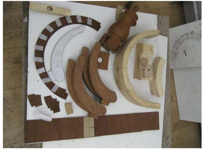
The hoop substrate was built up using pine brickwork glued with hide glue. Upon curing of the glue the excess pine was planed away and the hoop was hammer veneered in mahogany using pearl glue.
