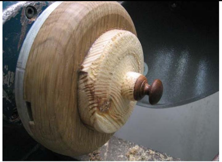
Three of the knobs had lost timber due to old breaks; the losses were filled with spliced in timber which was glued into place with hide glue before being re-turned on the lathe to match the original profile. After colouring with shellac and acrylics the knobs were re-fitted using pearl glue.
