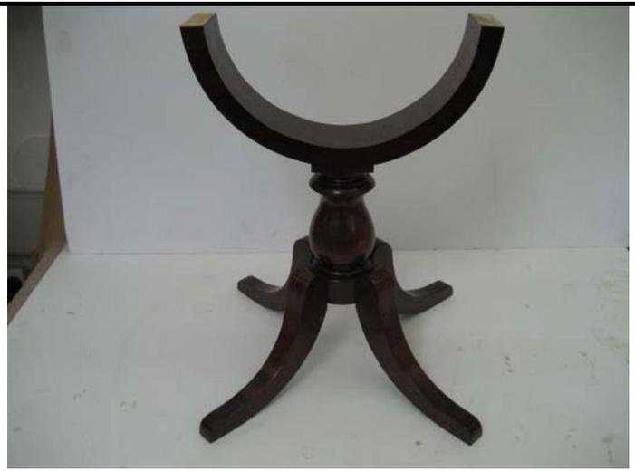
The taper was cut onto the legs and these were dry fitted to the column. The spacer was cut from mahogany and the finished hoop fitted into place. The replacement base was then sanded and stained using dichromate of potash, and adjusted for colour using proprietary bleaches and water stains before sealing with shellac. Final colour adjustment and gentle distressing was done using flint and water stains sealed into layers of shellac.
