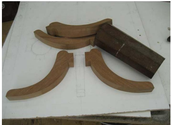
After agreement with the client work could begin; after research a 1:1 drawing was produced from which to work, templates were made and the legs cut out a prepared.
