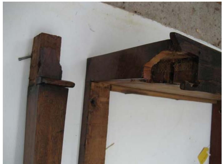
The Edwardian legs had been glued into place using hide glue – which was reversed using hot water injected with a syringe. The nail that can be seen in the photograph on the right was not visible until after the PL leg had been removed.
