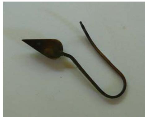
New spring bent to shape and 'aged'
