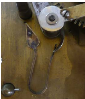
New spring fitted in place
